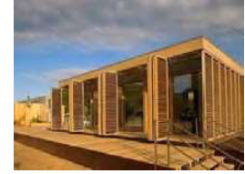
Kinetic shutters allow for shade in summer and solar gain in winter
